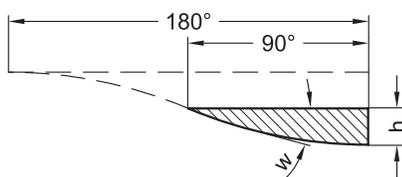
Looking at the developed view arising in an eccentric through the rolling motion, one will find that this is caused by a sinusoidal curve.
