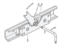
5. Turning the wrench clockwise presses the guide roller against the support raceway of the rail so that there is no play for the roller carriage. Overtightening will increase friction and reduce the service life of the item.
