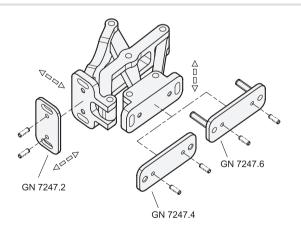
Multiple-joint hinges can be adjusted in three planes during installation. For example, this allows compensation for tolerances or establishing of required compressive forces for seals.
