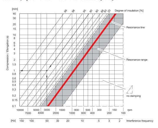
Example with the following assumptions: Disturbing frequency = 50 Hz; load = 120 N; desired degree of isolation = 90 %
