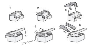
Prior to installation, remove the slam latch cover as shown in the sketch. Socket cap screws DIN 912, hex head screws DIN 933 and hex nuts ISO  $4032\ each$  with thread size M  $6\ can$  be used for mounting the slam latch.
