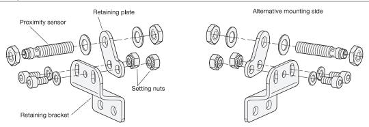
Sensor holders can be mounted on the left or right of the toggle clamp. To do this, the setting nuts must be tightened on the left or right of the retaining plate, to secure them against rotation and loss. This facilitates the further assembly of the sensor holder and the adjustment of the sensor. Subsequent changing of the mounting side is not intended.
