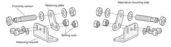
Sensor holders can be mounted on the left or right of the toggle clamp. To do this, the setting nuts must be tightened on the left or right of the retaining plate, to secure them against rotation and loss. This facilitates the further assembly of the sensor holder and the adjustment of the sensor. Subsequent changing of the mounting side is not intended.
