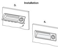
The recess in the door for mounting the cam latch / cam lock with gripping tray must be cut as shown in the outline drawing.
