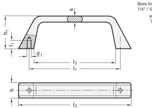
Bore for socket cap screw 1/4" / 5/16" or ISO 4762-M6 / M8
