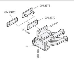
Multiple-joint hinges can be adjusted in three planes during installation. For example, this allows compensation for tolerances or establishing of required compressive forces for seals.
