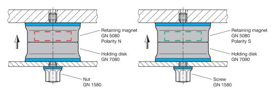
A normal holding force is achieved by combining retaining magnets with holding disks. Retaining magnets with north or south poles on the holding surface can be used equally.
