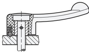
EN 623 / EN 623.5 control lever with ball and spring mechanism for indexing the positioning angle, attached with a cross pin. The cross pin is to be attached at an angle of 45° to the shaft axis. These parts are not included and must be ordered separately.
