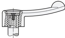
EN 623 / EN 623.5 control lever attached via a key / keyway, using a GN 184 countersunk washer (→ page 552).
