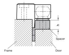
For applications with differences in height between frame and door, EN 450.1 spacer with height  $h=5\ mm$ , 10 mm and 15 mm are available.
