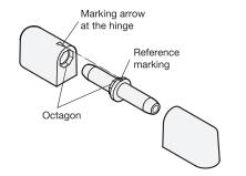
The eccentric pin is to be placed in eight positions via the octagon. Depending on position,  $I_1$  changes: min. 27.5 / max. 28.5 mm.
