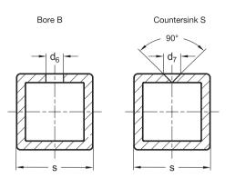
The square dimensions of these flanged connector clamps are designed for GN 990 construction tubes. These can be fitted by the user with locating holes (B or S) according to the dimensions specified in the table.
