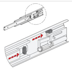
The rubber stops dampen the impact of the slide in the two end positions. This feature minimizes noise development and increases the service life. Attached to the slides in a partially concealed, partially visible manner, the stops meet each of the requirements in regards to shape, material, and hardness.
