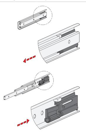
GN 1424 telescopic slides have a dampened self-retracting mechanism, which is also called "soft-close". The dampened self-retracting mechanism is divided into two main functions and provides the best possible ease of use when closing the extension.
