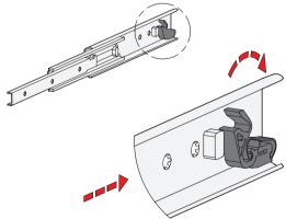
GN 1422 telescopic slides have an integrated self-retracting mechanism, which significantly improves the ease of use when closing the extensions.
