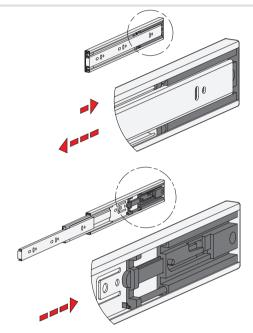
GN 1418 telescopic slides have an opening mechanism, which is referred to as "Push to Open" or "Touch to Open" mechanism. In addition to the best possible ease of use when opening an extension, this system offers the advantage to have drawers without a handle on the front side. This results in a simple and high-quality design.
