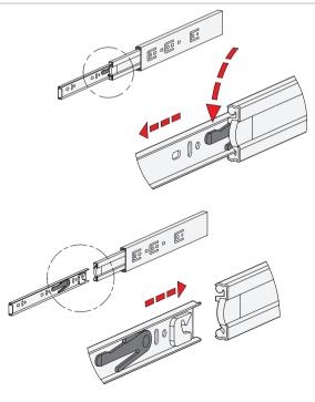
The detach function allows the extension to be completely separated from one another in the area of the middle and inner slide. This feature not only facilitates mounting, it also allows the extension to be quickly removed, for example when frequent maintenance work is performed on the components located behind.
