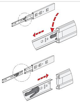
The detach function allows the extension to be completely separated from one another in the area of the middle and inner slide. This feature not only facilitates mounting, it also allows the extension to be quickly removed, for example when frequent maintenance work is performed on the components located behind.
