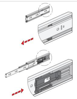
GN 1414 telescopic slides have a dampened self-retracting mechanism, which is also called "soft-close". The dampened self-retracting mechanism is divided into two main functions and provides the best possible ease of use when closing an extension.
