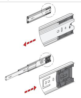
GN 1412 telescopic slides have an integrated self-retracting mechanism, which significantly improves the ease of use when closing the extensions.
