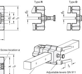
Construction tube with locating holes GN 990.1
