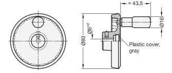
Flat-Faced Solid Disk Handwheel for
