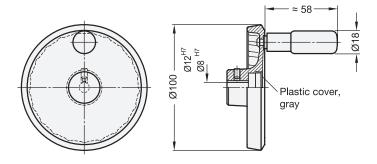
Flat-Faced Solid Disk Handwheel for
