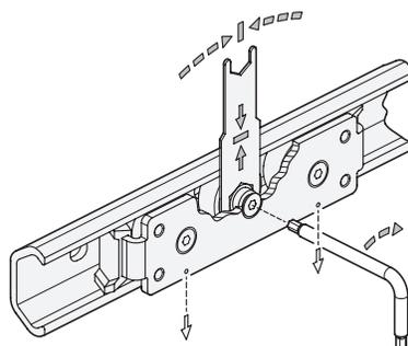
7. Move the cam roller carriage in the guide rail and make sure that the play or slight preload is consistent across the entire length of the rail. The cam roller carriage should move easily without being overly loose or tight. Adjust if necessary.
