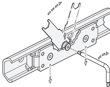
5. Turning the wrench clockwise presses the guide roller against the support raceway of the rail so that there is no play for the roller carriage. Overtightening will increase friction and reduce the service life of the item.
