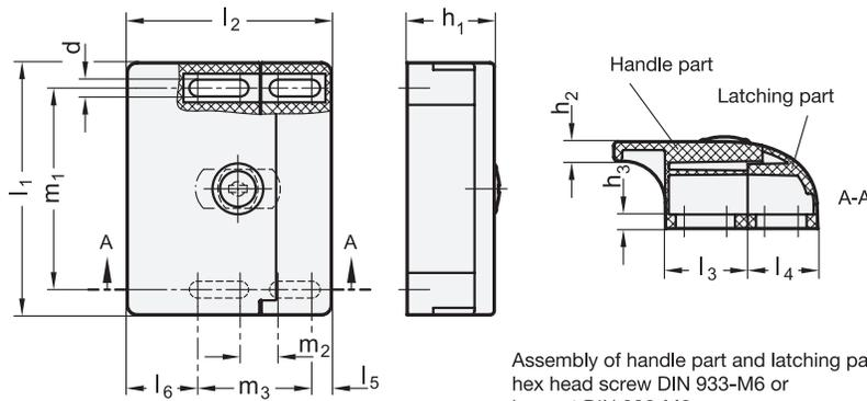
Assembly of handle part and latching part with hex head screw DIN 933-M6 or hex nut DIN 936-M6
