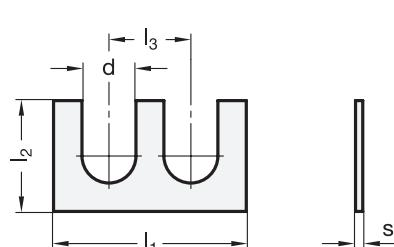
Gripper jaw block brackets GN 868 (Type R)
