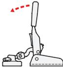
Lift the lever arm until the latch bolt is disengaged from the catch.
