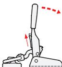
The latch bolt engages with the catch if the safety locking mechanism is moved upward during clamping. When clamping in the end position, the system locks automatically by spring force.
