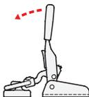
For **clamping**, lift the lever arm until the latch bolt rests on the catch.
