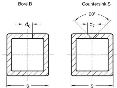
The square dimensions of these flanged connector clamps are designed for GN 990 construction tubes. These can be fitted by the user with locating holes (B or S) according to the dimensions specified in the table.
