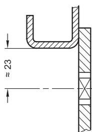
**Installation hole for punching or laser machining**
